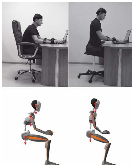
Fig. 4. The location of body segments in various sitting positions while sitting in a standard office chair (left image) compared to our anatomical chair prototype (right image)
